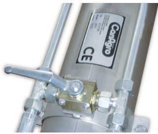
OPERATION VIA SHUT-OFF VALVE
