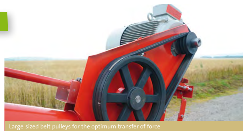
Large-sized belt pulleys for the optimum transfer of force
