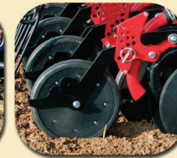
Press wheel with fertilizer supply
